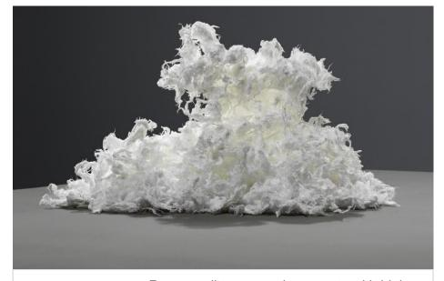
Re:newcell turns used garments with high REDEWCELL cellulosic content (e.g. cotton) into biodegradable raw materials to make clothes.
